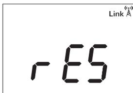
To confirm the reset of the unit, press **OK/Mode** button, to cancel it any other button can be pressed.
