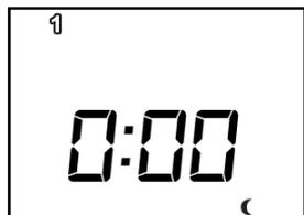
**3.2.3** Now the hours start to flash. Press the "+" and "-" button until you reach the correct time (hour) and Press the **OK/Mode** button.
