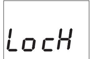
To unlock the keyboard, press the “+” and “-” buttons simultaneously for 3 seconds.
