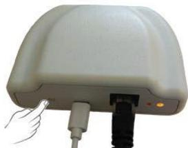
**4.2** With the hub in discovery mode, press the **Ok/Mode** button on the heater for 3 seconds until the Link symbol is shown.
